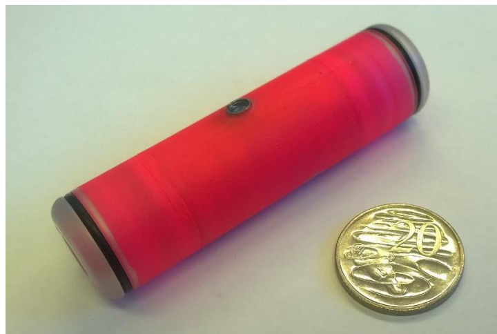
Figure 1. The Sensor Fish device with Australian 20 cent piece for scale. Pressure sensor is visible at the top centre of the Sensor Fish, and high visibility red paint was applied to aid in recovery after deployment.
