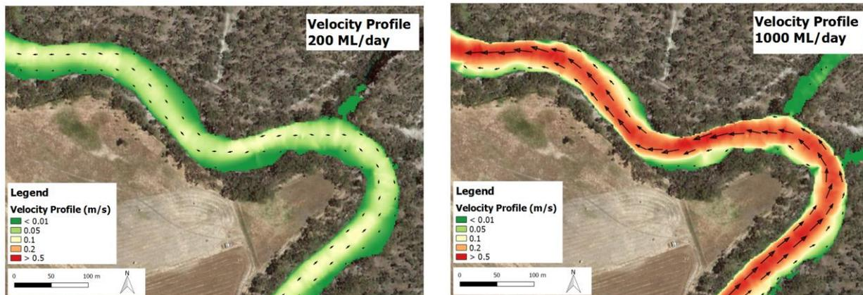
**Figure 2 – Velocity profiles generated from the 2D model in Reach 4 of the Lower Broken Creek. The model outputs show that a flow rate of 200 ML/d (left) would be unlikely to generate sufficient velocities to mobilise azolla whereas a flow rate of 1,000 ML/d (right) would be more successful in achieving this objective.**
