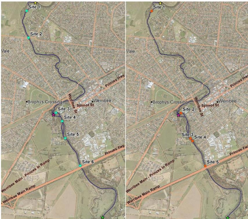
Figure 4. Location of ADCP Transects for 20 ML/d (left) and 200 ML/d (right) Flowrate Events
