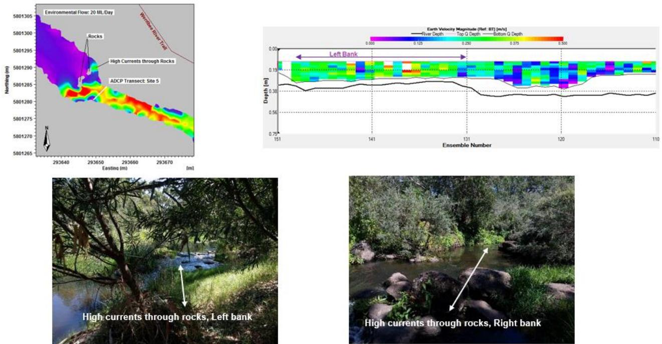
Figure 6. Modelled Velocities (left) and ADCP Transects (Right) for the 20 ML/d event at Site 5
