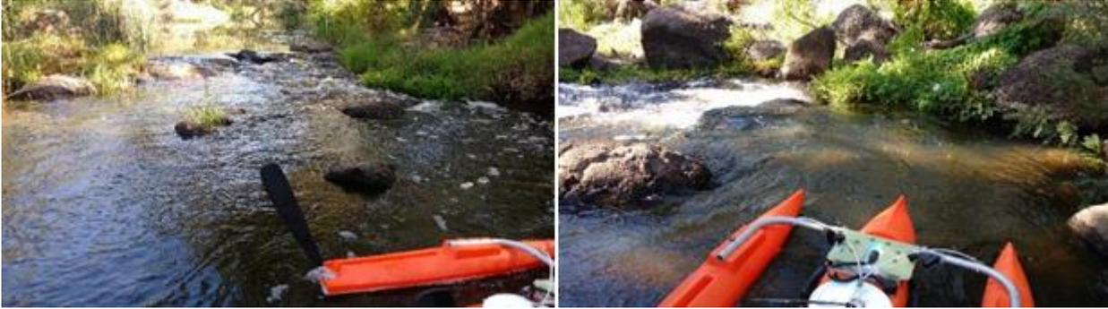
Figure 3. RiverPro ADCP, measuring velocities in Werribee River
