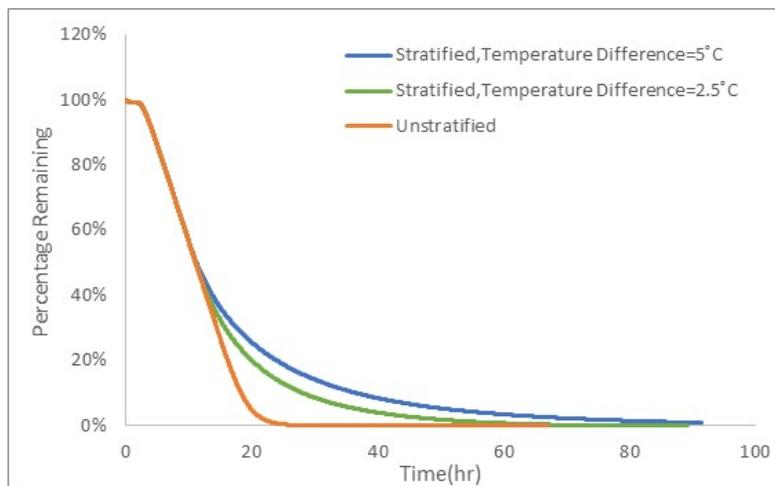
**Figure 8. Flushing conditions under stratified and unstratified conditions for the 3D model: 100 ML/d**
