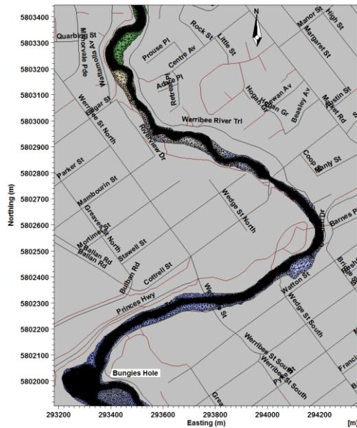
Figure 5. Model Mesh in Reach 2
