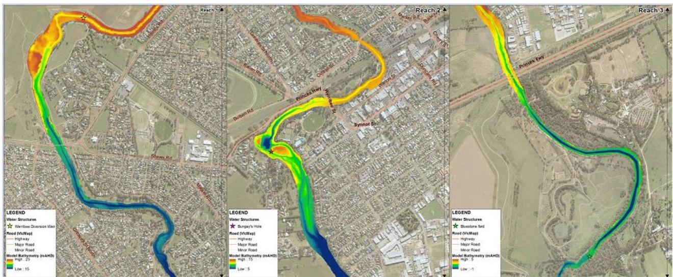
Figure 2. Model DEM in Reach 1 (left), Reach 2 (middle) and Reach 3 (right) of Lower Werribee River
