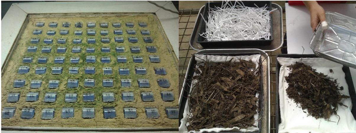
**Figure 1.** Thermogradient plate used to assess optimal temperature (left) and an example of the leaf litter trays used to assess seed application and litter presence and depth (right).
