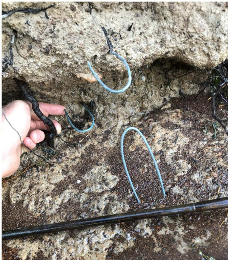
Figure 4. Erosion pins located at water level, 10cm above water level and 20cm above water level. Note the erosion of 1.1cm behind the middle pin in the photo (located at 10cm above water level).
