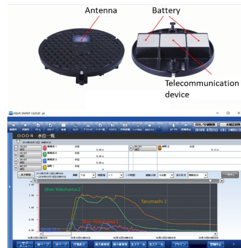
Figure 6. Smart Manhole cover (upper figure) for real-time sensing of water level in sewer networks to be seen over the internet cloud system (lower figure)
